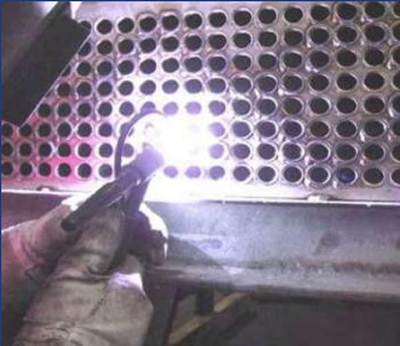
Hàn ống Tube/Tube welding work
