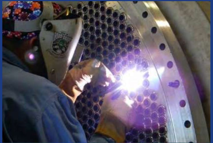
Hàn ống Tube/Tube welding work
